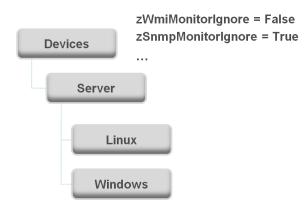
At the root of the device hierarchy is the Devices object. All device class configuration properties are defined here. Their values are the default values for the entire hierarchy.
