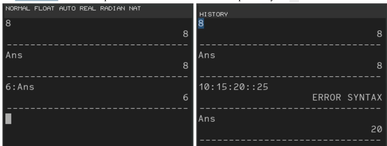
Manual assignment of a variable `Ans` (including attempts to modify list or matrix elements) will result in an [\*\*READ ONLY VAR\*\*](#) error. Assigning a list value to the variable `Ans`, as well as using the construct `<Size:Dec>→dim(Ans)`, will lead to the creation or modification of the variable `Ans`. Assigning a matrix value to the variable `Ans`, as well as using the construct `<Height, Width:List>→dim(Ans)`, will lead to the creation or modification of the variable `[Ans]`.
