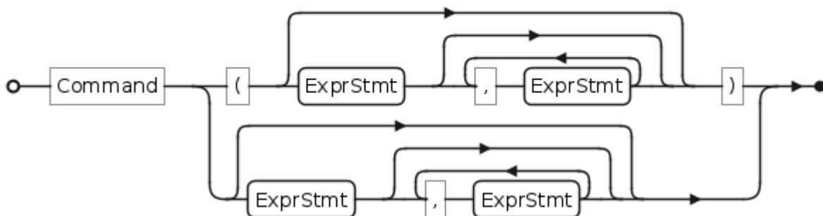
The marker for analyzing CommandStmt is the [Command] token. Mismatch in the following syntax will lead to an error.
