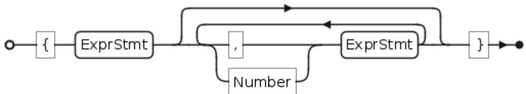
The [Number] token is included in the subsequent ExprStmt node. This analysis structure allows for the following syntax in the script file:
