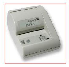
This reading process is called Magnetic Ink Character Recognition (MICR). The main advantages of MICR are that it is fast and less error prone.
