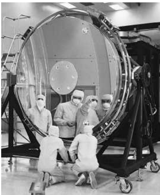
The 2.4-m-diameter hyperboloidal primary mirror of the Hubble Space Telescope. (NASA)
