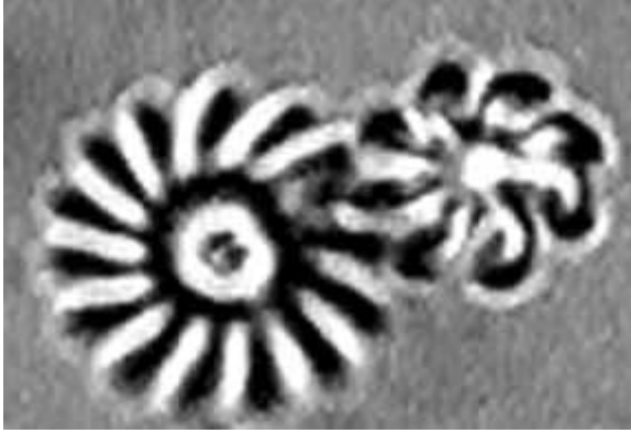
Two tiny pinwheels about 5 μm in diameter (that’s roughly only 1/15 the width of a human hair). These microscopic gears are so small they can be spun around by the pressure of a light beam. (Galajda and Ormos/Hungarian Academy of Sciences)
