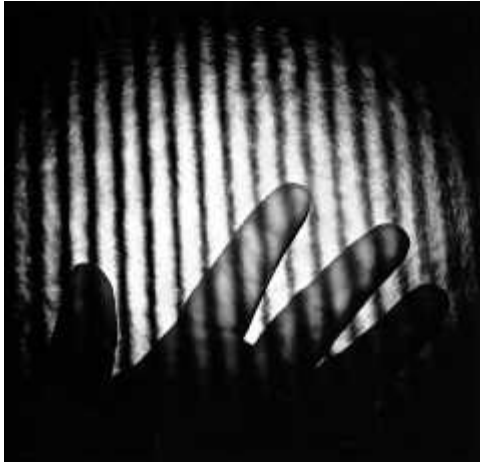
Real Michelson fringes using He–Ne laser light. (E.H.)
