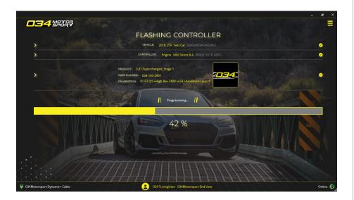
15. **Please Note:** During the flashing process, you will encounter multiple warnings/lights on the dash from various systems. This is completely normal and will be resolved at the end of the flash.
